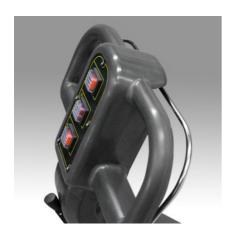
User friendly analog control panel. Control lever for brush operation and detergent water outflow.
